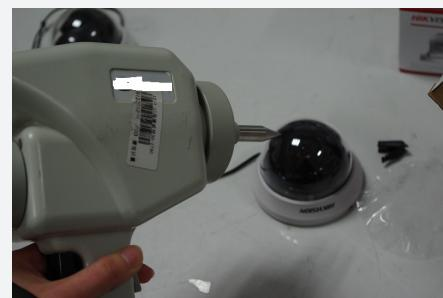
Test device for electrostatic discharge anti-interference
